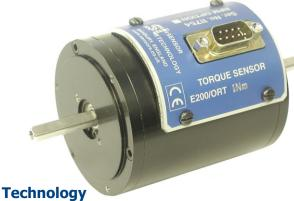
An extensively developed measurement principle is used, in which the intensity of light beams is measured by means of photovoltaic detectors, and the electrical output is used to provide precise indication of the applied torque transmitted by the shaft.
