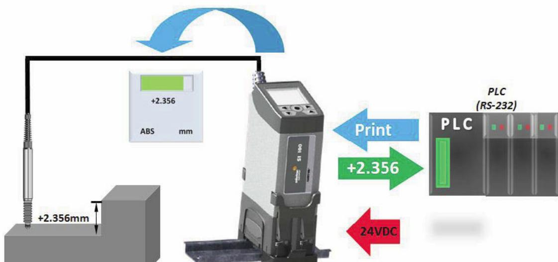
FROM MEASUREMENT SI100 to PLC USING PRINT INPUT AND RS-232 SERIAL PORT
