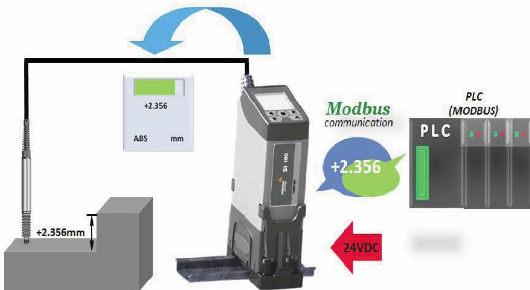
FROM MEASUREMENT SI100 to PLC via MODBUS
