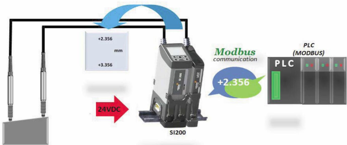
FROM MEASUREMENT SI100 to PLC USING PRINT INPUT AND RS-232 SERIAL PORT
